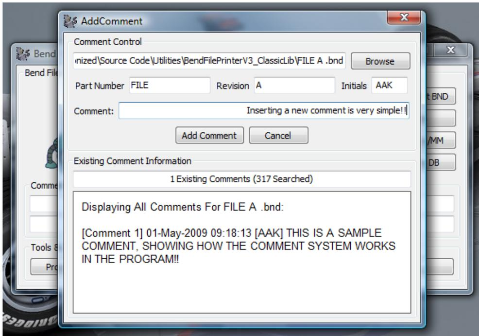
Inserting comments into the database is very simple. If an existing BND/DAT/FLX is loaded, most of the data is set up for you. Comments are stored on a per-revision basis unless the global wildcards are used. The screen also displays any existing comments, so you are not duplicating anything!
