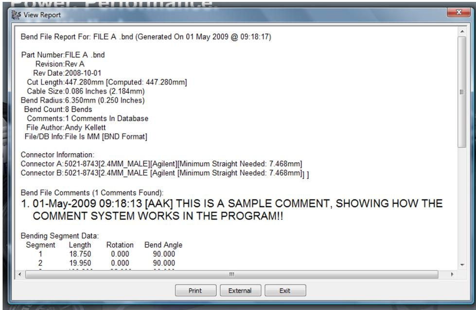
Viewing the single BND cable report. In this example, the comment is shown in bold uppercase letters. Errors found in the cable design are also shown in the same way to alert them to an operators attention.
