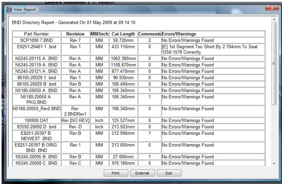
This is the same built-in report viewer, after selecting an entire directory for processing. Each file analyzed is listed, and any errors/warnings detected are listed in the table for easy viewing/printing. Non-compatible files such as CAD/PDF files are automatically skipped. These reports can be attached to emails as well.
